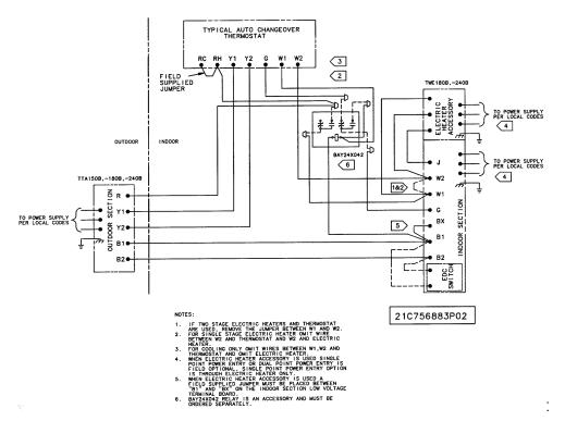
Figure 23. TTA150B, 180B, 240B/TWE 180B, 240B; TTA125B, 155B, 200B/TWE155B, 200B; TTA155C/TWE155B; TTA180C/TWE180B
